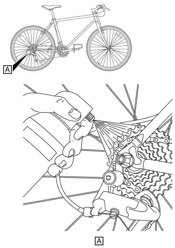
ICN-S1000DBIKE-AAA-DA52000-0-U8025-00523-A-04-1 Fig 2 Degreasing the freehub
